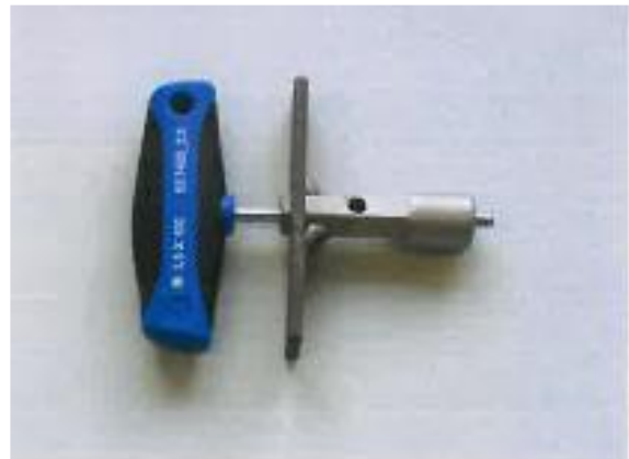
Figure 20 T-720 Wrench, Governor Adjusting
