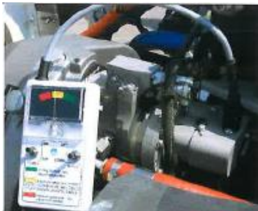
Figure 19 T-719-A Governor Test Box
