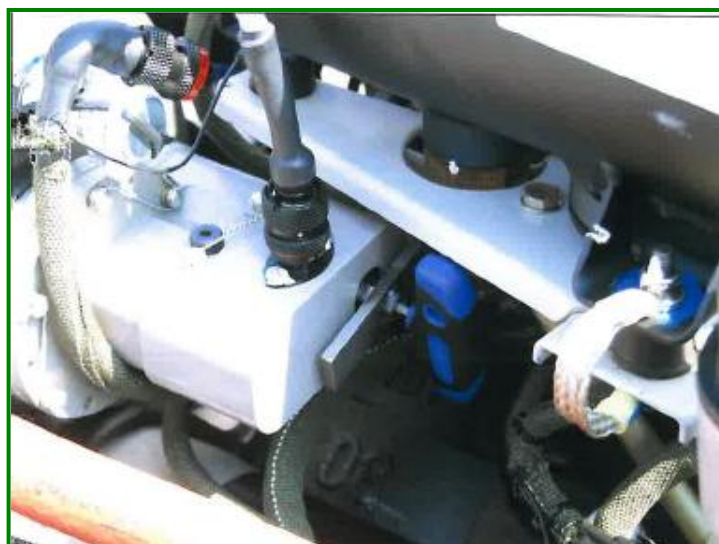
Figure 22 Using T-720 wrench
