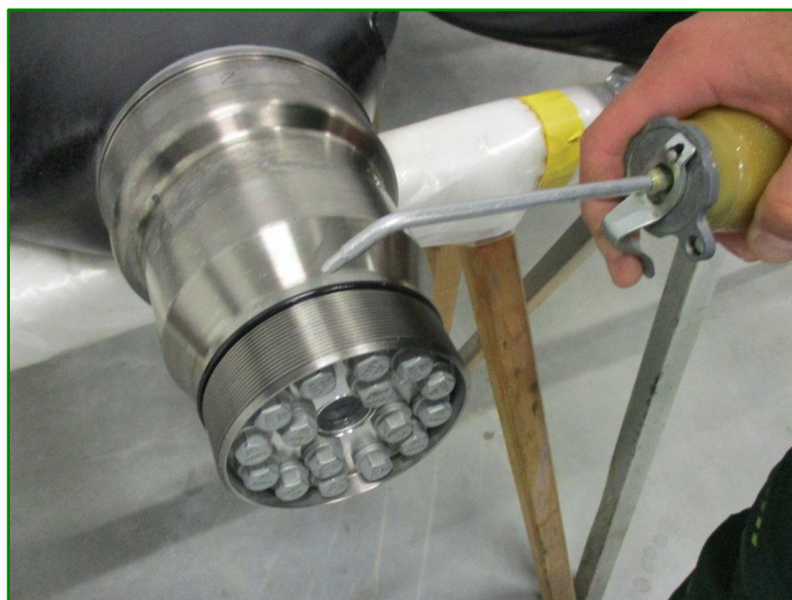
Figure 1: Lubricated O-Ring and thread on the blade ferrule
