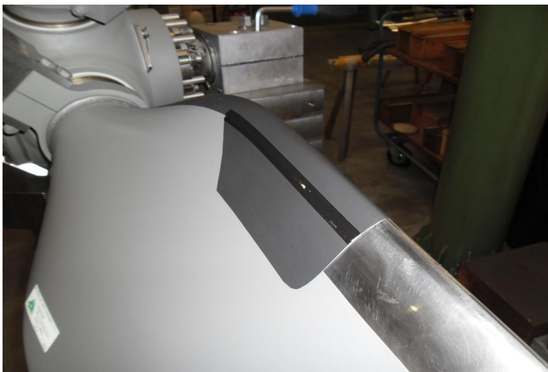
[7] Finished installation of the Protective PU Tape Blanks
