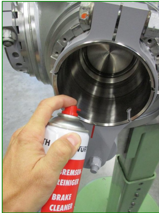
Figure 2: Cleaned degreased surface.
