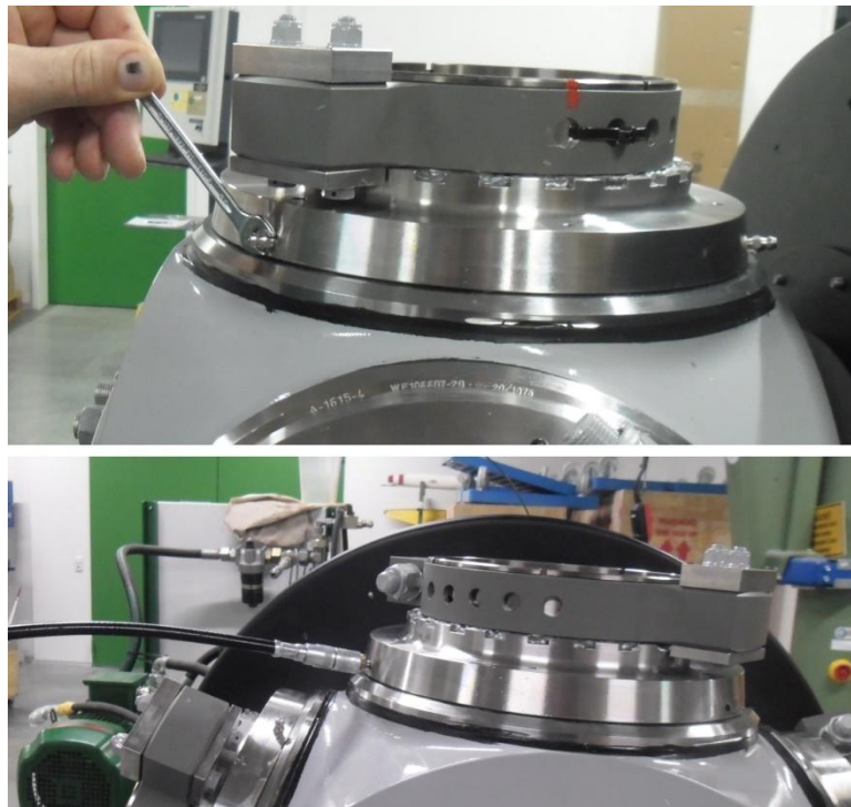
Figure 14: Removal of one grease fitting and application of grease
