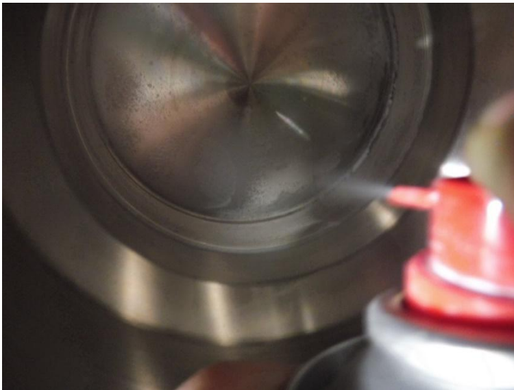
Figure 5: Lubricate inner thread with PTFE dry lubrication spray
