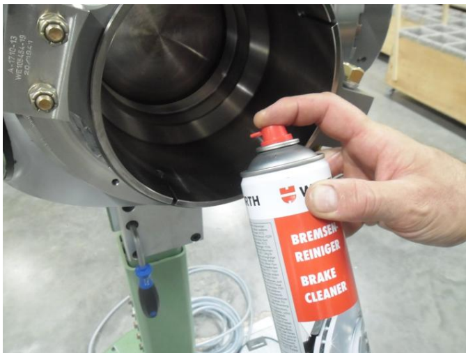
Figure 6: Cleaned and degreased surfaces, used for clamping for the friction to fix the inner blade in the outer blade ferrule
