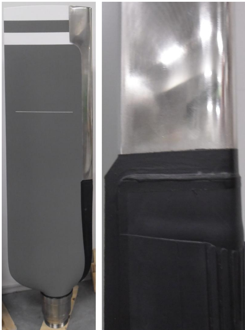
Figure 19: Blade with boots in root area
