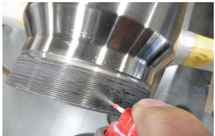
Figure 4 / 4a: Lubricate the thread on the blade ferrule only with PTFE dry lubrication
