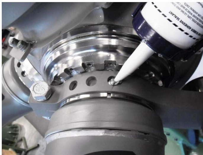
Figure 9: Seal the unused bores with silicone RTV 109
