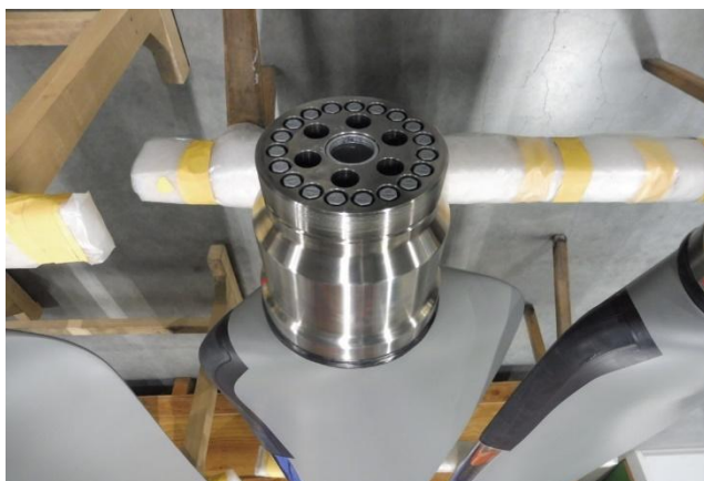
Figure 4 / 4a: Lubricate the thread on the blade ferrule only with PTFE dry lubrication
