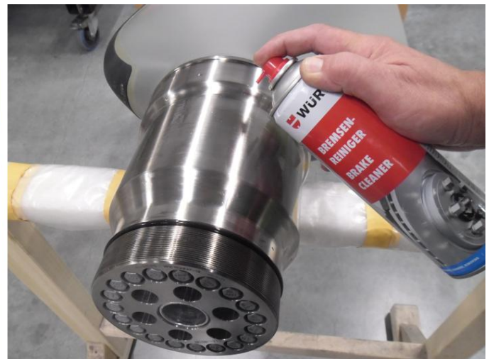
Figure 6: Cleaned and degreased surfaces, used for clamping for the friction to fix the inner blade in the outer blade ferrule
