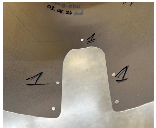
Figure 4: Marking of blade 1 inside spinner dome
