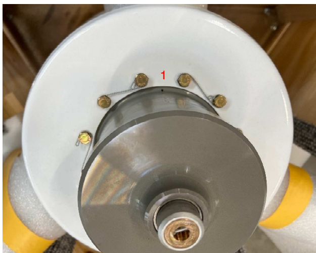
Figure 3: Marking of blade 1 on spinner front plate
