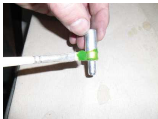
Figure 7: Apply Hysol EA 9359.3 at the bigger diameter of the pitch change pin
