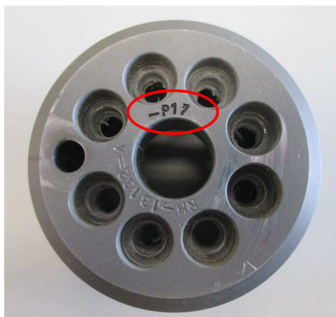
Figure 5: Blade ferrule marked with “-P17” for replacement of the pitch change pin in the year 2017
