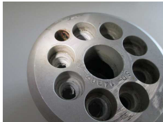
Figure 4: Corrosion in blade ferrule bore for pitch change pin
