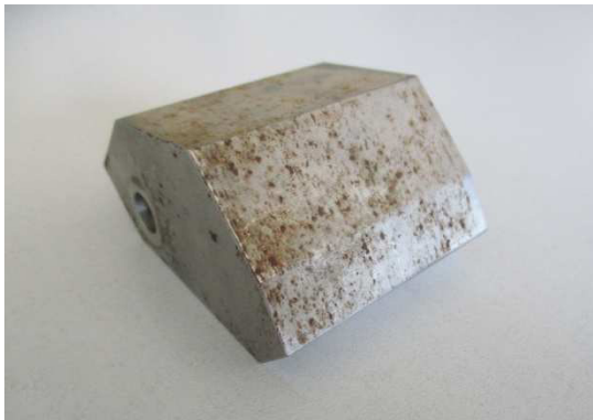
Figure 1: Corrosion on counterweight module
