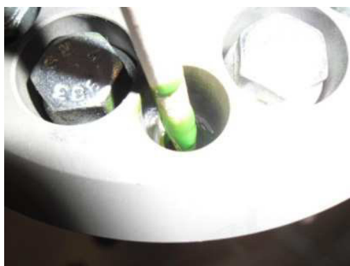
Figure 6: Apply Hysol EA 9359.3 in the inner bore of the blade ferrule
