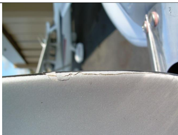
Longitudinal cracks may be sealed with 5-Minute Epoxy
