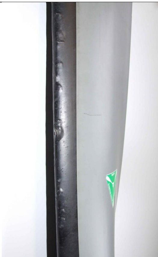
Typical Damage: Punched through PU-Strip
