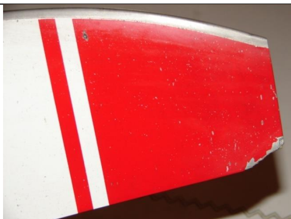
Hangar Damage: Broken Tip Trailing Edge Seal with 5 Minute Epoxy or permanent repair with Fiber Glass.
