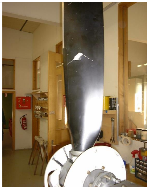
Blade surface damage obviously exceeding the field repair limits
