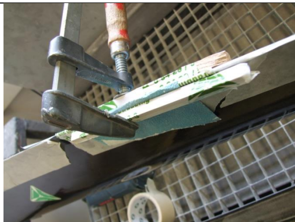
Then clamp the trailing edge with C-clamps and let the epoxy cure. Then clean the trailing edge and repaint the repaired areal.
