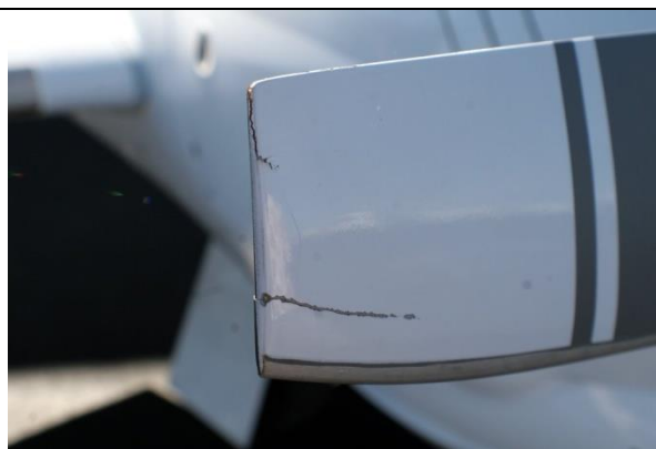
Split Blade Tip and delaminated trailing Edge. Rebond Trailing Edge with 5 Minute Epoxy. Repair split Tip with Fiber Glass
