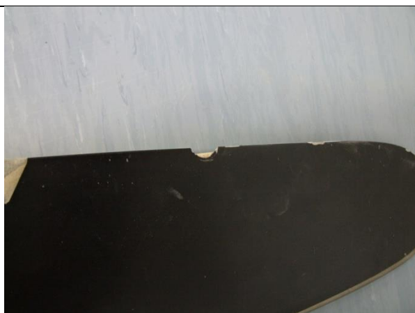
Minor damage on the trailing edges may be sealed with 5-Minute Epoxy
