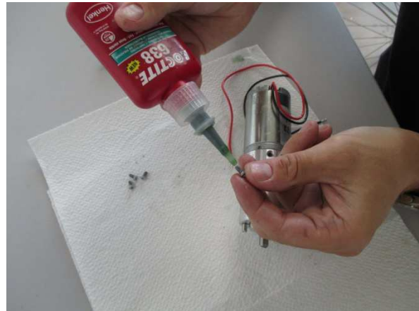
17) Secure and bolt on the screws (hand tighten) with Loctite
