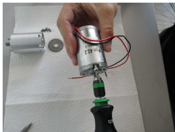
9) tighten this screw by hand only
