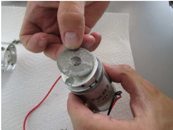
4) remove spacer between gearbox and motor
