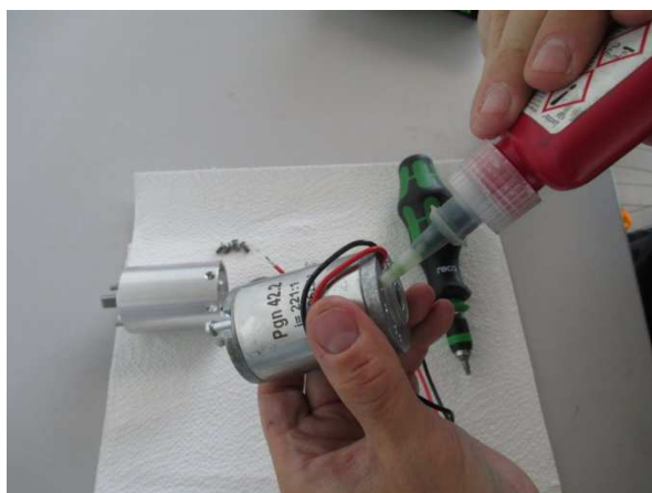
8) put Loctite in the threaded hole, not on
