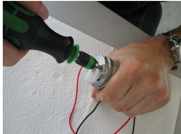
5) unscrew the two cover screws of the motor
