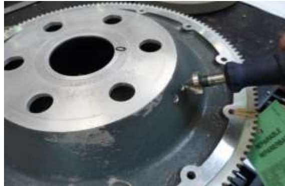
4) Deburr the holes on both ends
