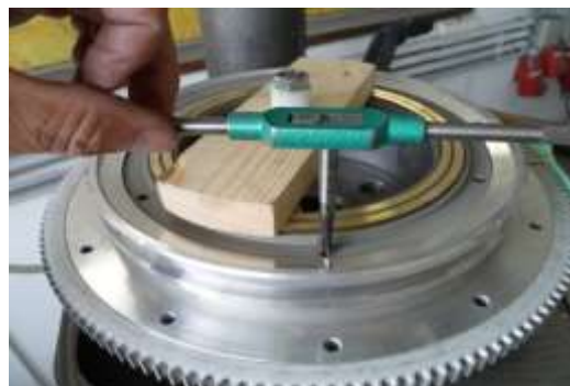
8) For the thread use the \frac{1}{4} "-28 UNF tap
