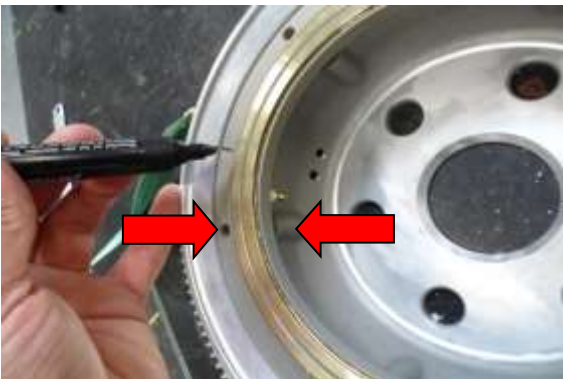
5) Position the slip ring that the starter gear aligns with the holes
