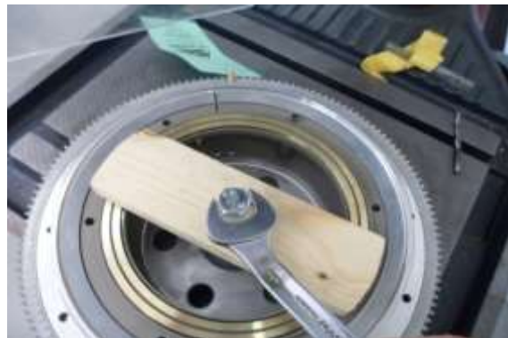
6) Fix the slip ring into the starter gear with the self made clamp tool
