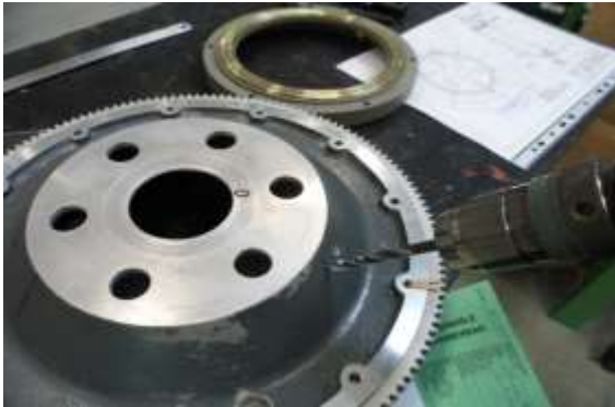
3) Bore two holes with a \varnothing 6,0\text{mm} (0,236") drill
